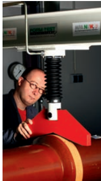
Realistic testing of sleeve joints
