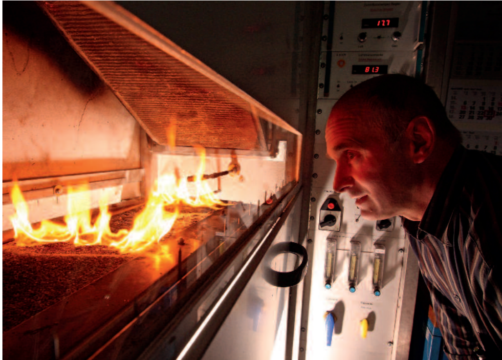
Testing the fire behaviour of floor coverings with the "Radiant Panel Test" according to DIN EN ISO 9239-1 or DIN 4102-14
