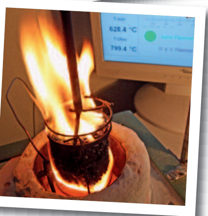
European test procedure "non-combustibility furnace" according to DIN EN ISO 1182
