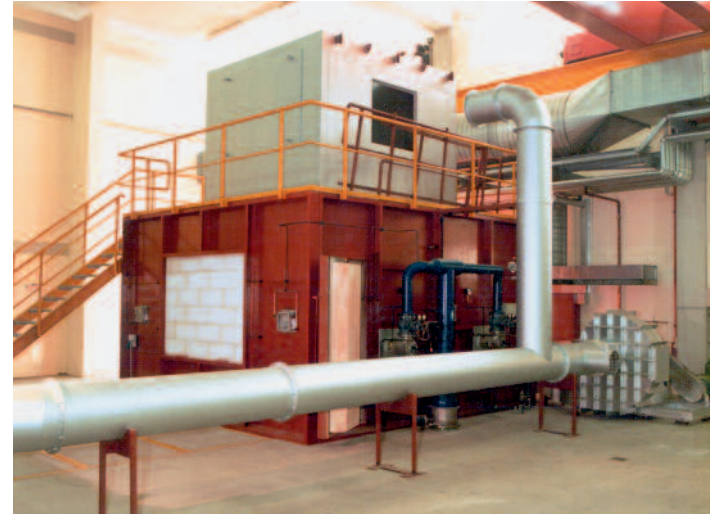
The only furnace in Germany according to DIN 4102-6 for testing horizontal and vertical ventilation ducts
