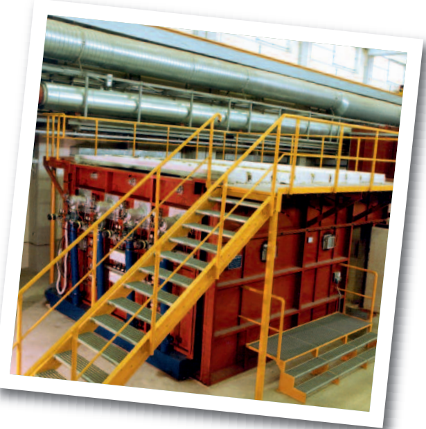
Multifunctional furnace with gas flame treatment for European tests on vertical and horizontal components
