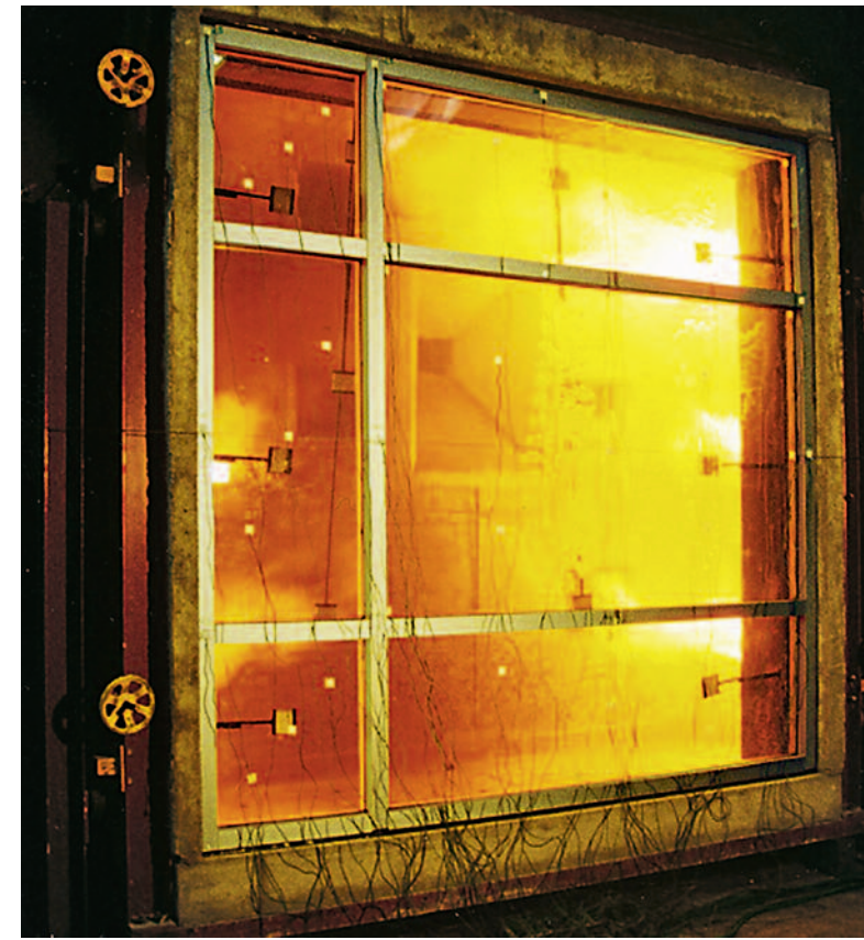
Shortly after the start of a fire test with oil flame treatment on a glazing of 3 x 3 metres
