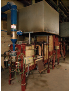
Two furnaces according to DIN 4102-8 comparison and surveillance tests
