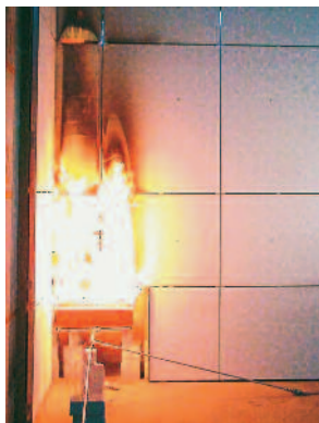
Large-scale test in actual size for wall cladding elements
