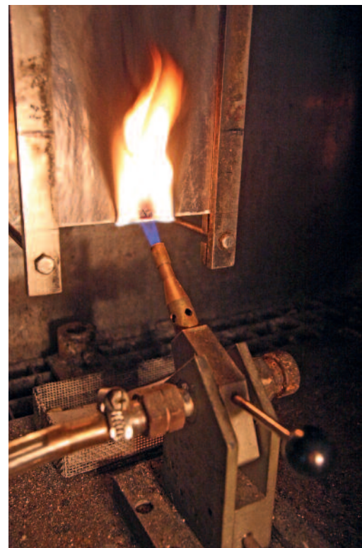
Ignitability test according to DIN EN ISO 11925-2 or DIN 4102-1, building material class B2
