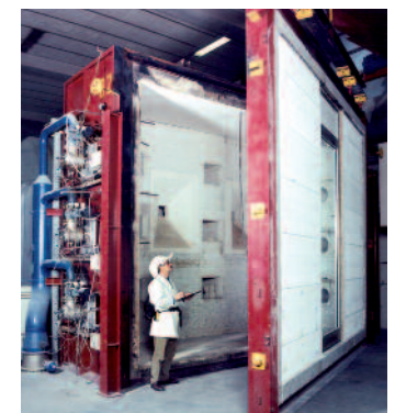
Checking a 5 metres wide and 4 metres high test specimen before the fire test
