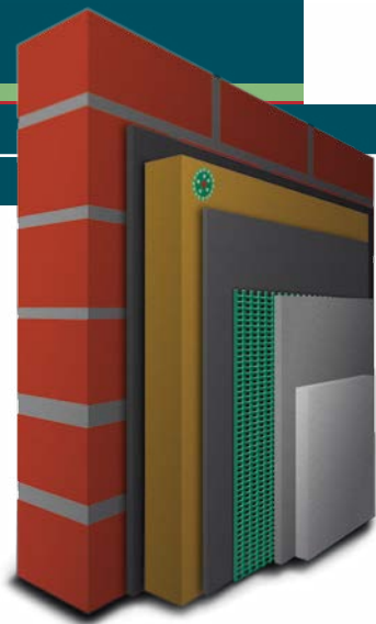
External thermal insulation composite systems (with rendering) consist of various components: insulation, reinforcement, rendering and attachment.
