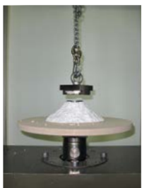
insulation sample (EPS) after a dowel pull test
