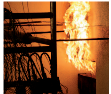
Testing the fire behaviour of composite heat insulation systems
