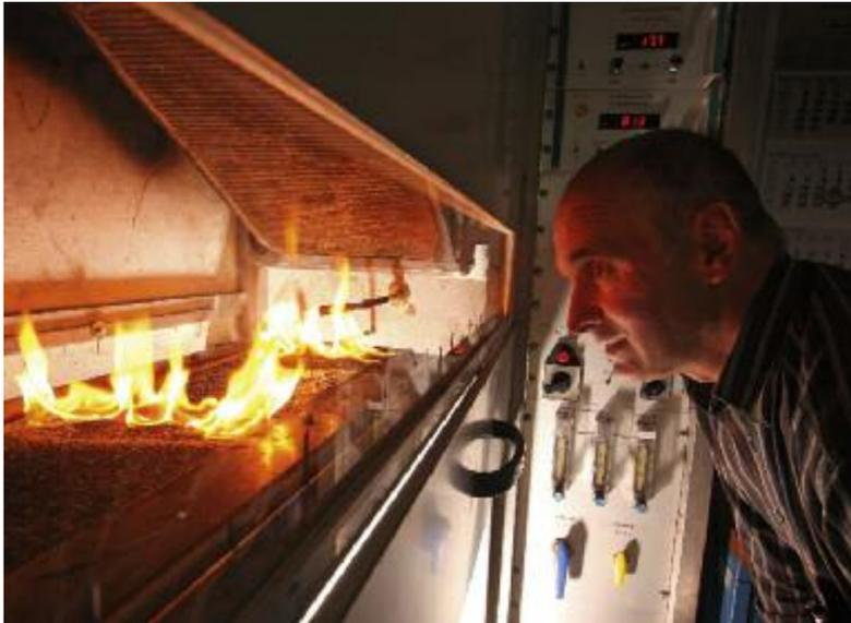
Testing the fire behaviour of floor coverings with the "Radiant Panel Test" according to DIN EN ISO 9239-1 or DIN 4102-14
