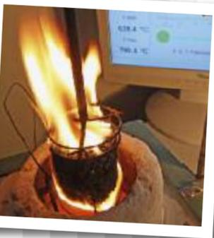
European test procedure "non-combustibility furnace" according to DIN EN ISO 1182
