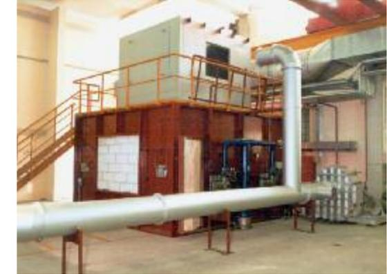
The only furnace in Germany according to DIN 4102-6 for testing horizontal and vertical ventilation ducts
