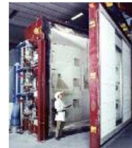
Checking a 5 metres wide and 4 metres high test specimen before the fire test
