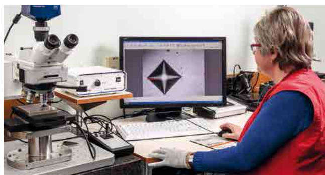
Measurement of a calibration indentation according to Vickers
