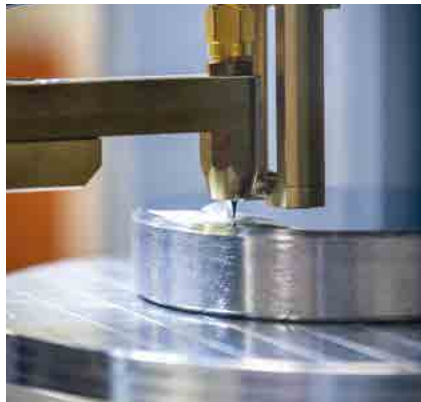
E-module determination on a hardness reference block for the UCI-procedure
