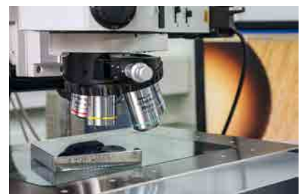
Measurement of a calibration indentation according to Brinell
