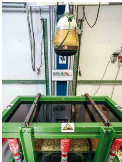
Headform test with deceleration measurement for determining the risk of injury of a passenger head hitting a plastic pane.
