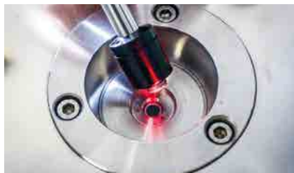
Calibration of a hardness tester according to Leeb
