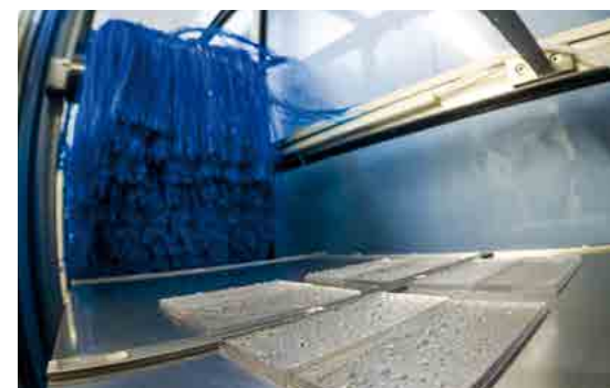
Car wash test for testing the abrasion resistance of plastic glazing
