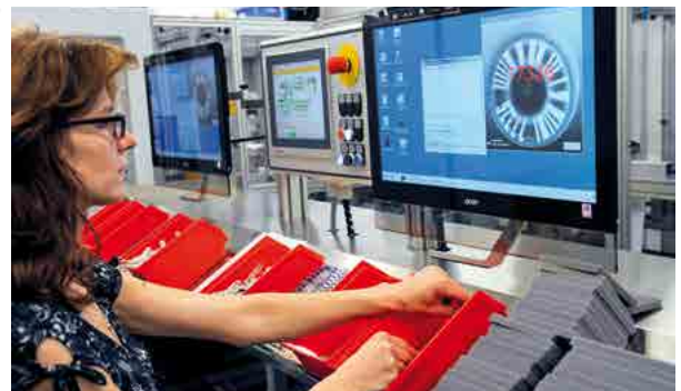
At a manual workplace e. g. ring dosimeters can be placed into the parcel.
