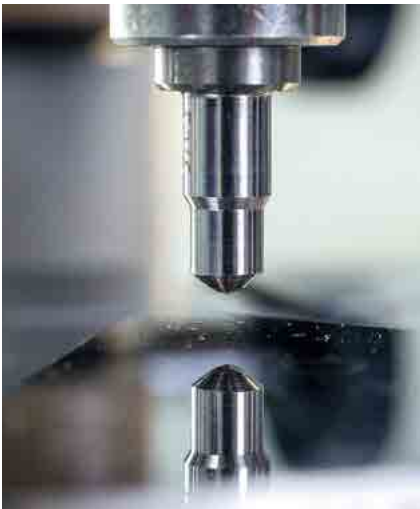
Vickers indenter approaching the surface
