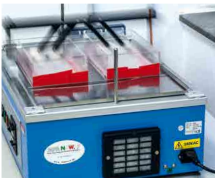
Device for determining the abrasion resistance by means of wiper test
