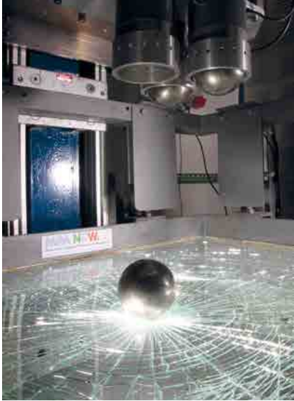
Ball drop test for determining the resistance against manual attack of architectural glass
