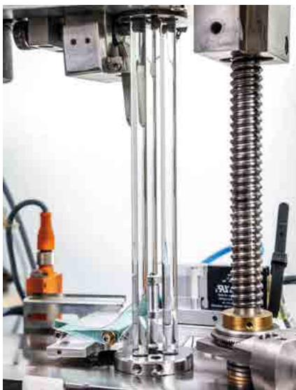
Falling body before hitting the surface during the calibration of a hardness reference block according to Leeb (left photo)
