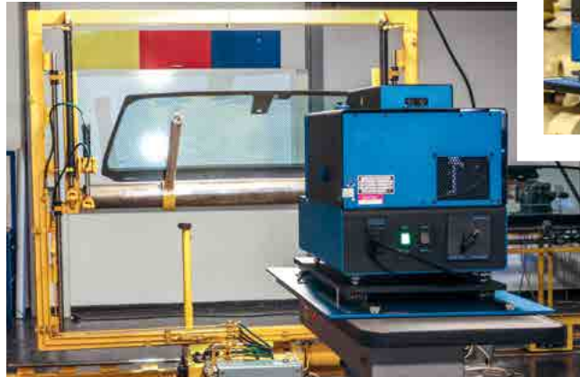
Large format projector for testing the optical properties of a windscreen by raster projection
