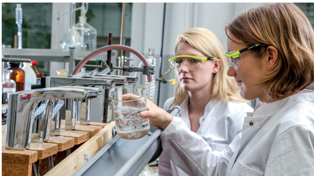
The apprentices as a chemical lab technician taking samples at the test stand for determining the migration of heavy metals
