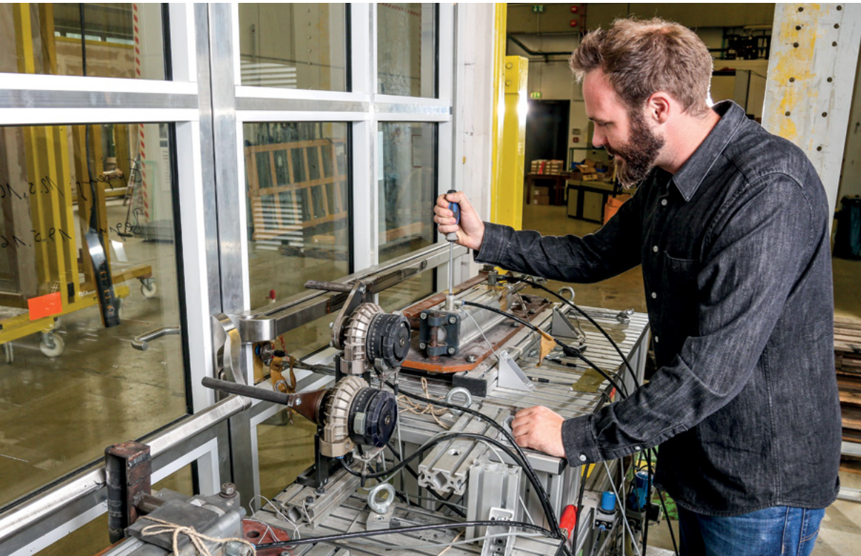
Durability test according to EN 1191
