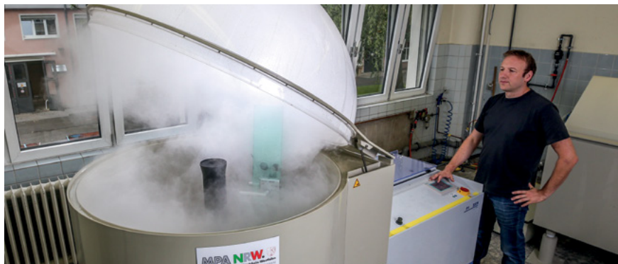
Salt-spray chamber according to DIN EN ISO 9227
