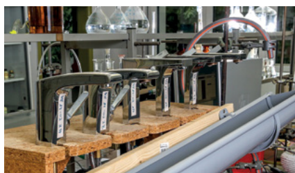
Lavatory taps in the test stand for determining the migration of heavy metals
